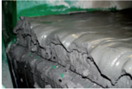
Dewatered solids discharge from Derrick High-g force linear motion shaker
